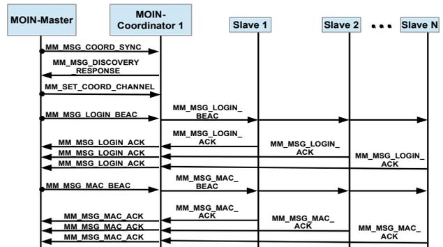
Fig. 6: Communication sequence realized by the MOIN Component Interaction Protocol
