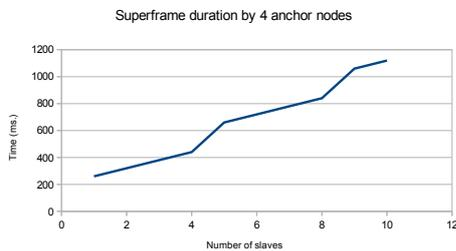
Fig. 9: Superframe duration with 4 anchors for localization
