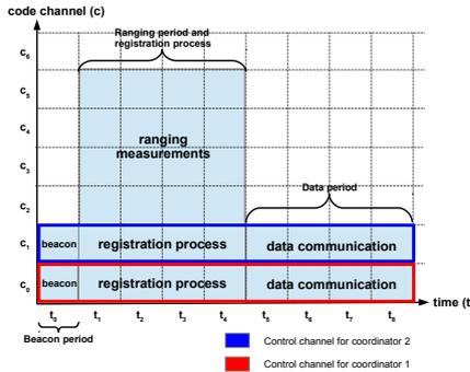
Fig. 5: Representation of the slot configuration in MOIN
