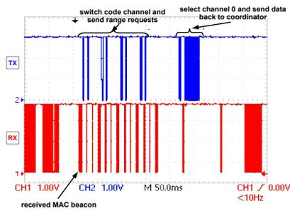
Fig. 8: Timing of a slave node with four ranging measurements
