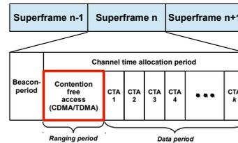
Fig. 4: Modified MAC superframe structure
